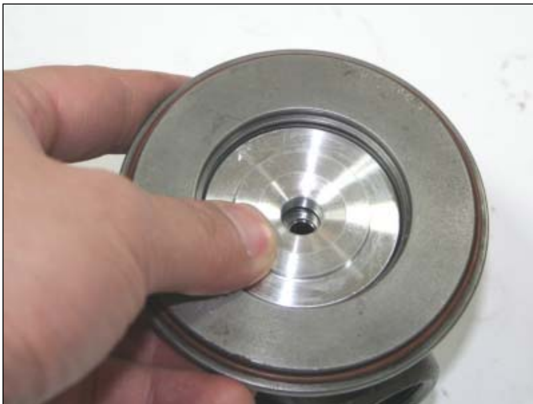
Push the carbon seal plate to the bottom
