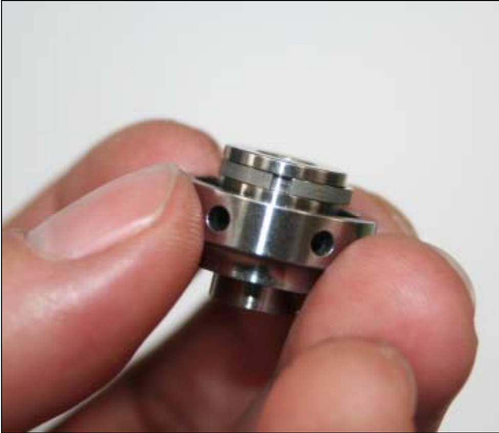
Piston Ring on thrust collar
