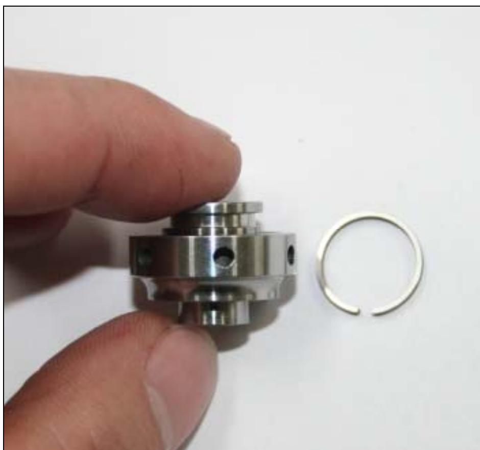
Press small piston ring into thrust collar
