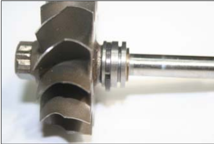
It is the turbine wheel / shaft with new piston ring
