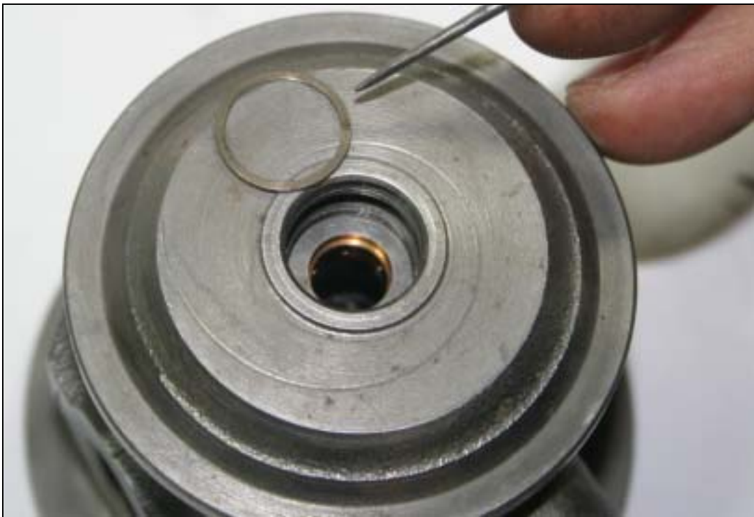
Another ring to fix the oil deflector and journal bearing
