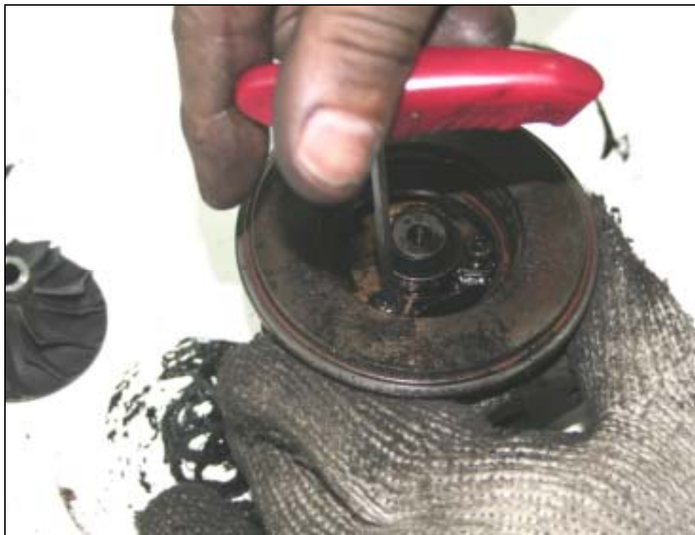
Remove the bolt and then you get the thrust bearing and collar
