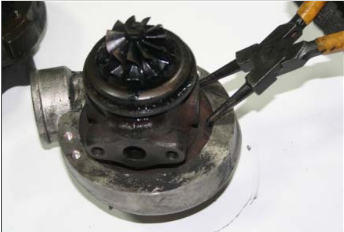
Remove the snap ring, and then you can see the CHRA and compressor housing
