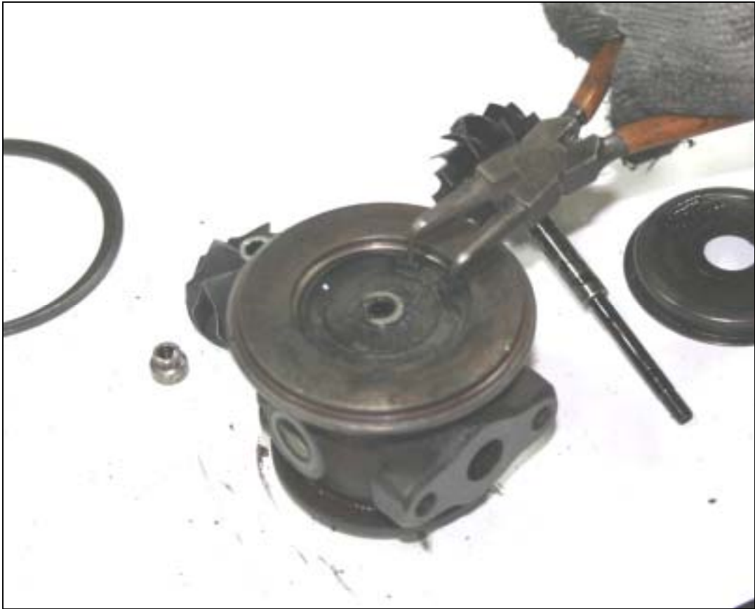
Remove the snap ring and seal plate
