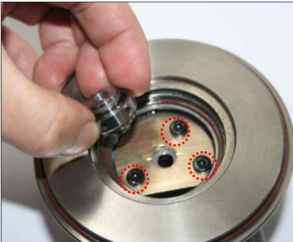
Bolt the thrust bearing before you install thrust collar
