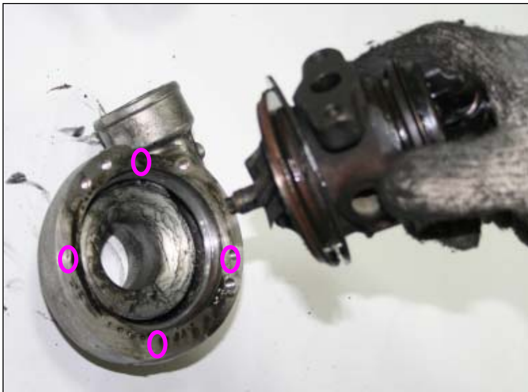
Remove the snap ring, and then you can see the CHRA and compressor housing
